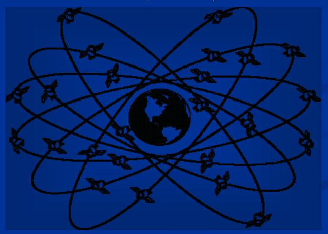
The distance (x) from one satellite tells us we're located somewhere on the surface of an imaginary sphere centered on that satellite with a radius of x.
