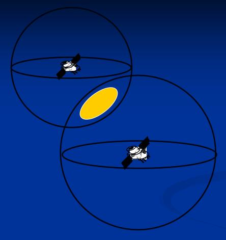
Distance measurements from two satellites limits our location to the intersection of two spheres, which is a circle.
